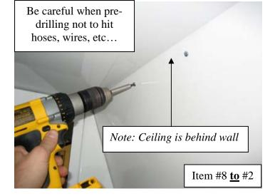
Pre-drill ceiling with 5/32" drill bit and attach #10 x 1" Phillips pan head sheet metal screws to hold **Ceiling** to **Bench/Wall** assembly. *Repeat these steps on the Passenger-side Ceiling section*
